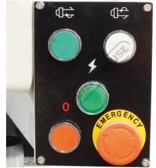
Horizontal Spindle Control Panel
