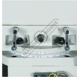
Adjustable Swivel and Sliding Ram
