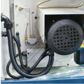
Oil Feeder Distribution Block
