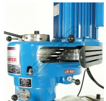
8 Speed V Belt Drive System
