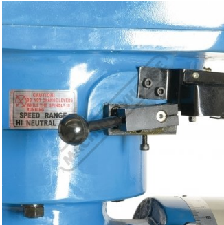
High Low Speed Range Selection Lever
