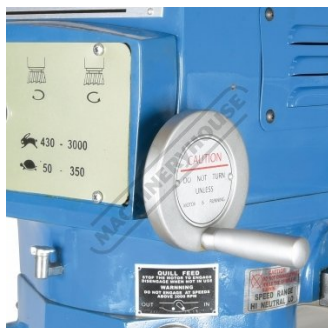
Variable Speed Hand Wheel
