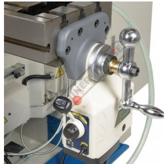
X Axis Power Feed with Rapid
