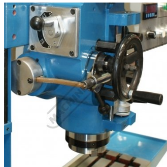
Quill Feed Mechanism
