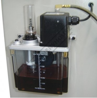
Auto Lubrication System
