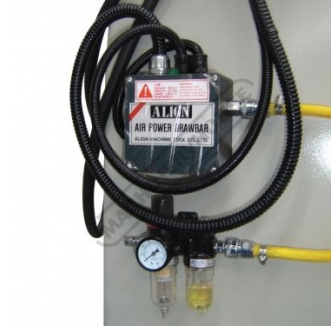
Align Air Operated Drawbar System
