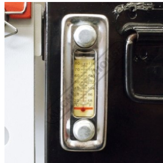
Hydraulic Oil Level Gauge
