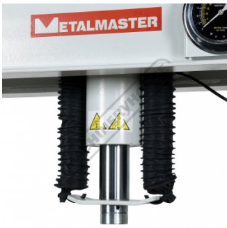
Ram With Safety Covers for Springs
