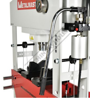
Manual Hydraulic and Pneumatic System
