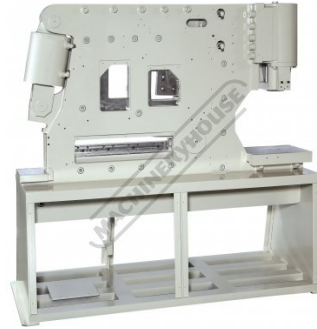
Monoblock Design For Rigid Frame Structure
