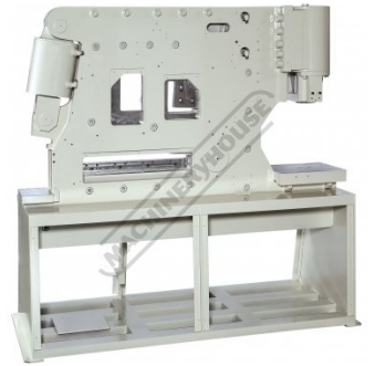
Monoblock Design For Rigid Frame Structure
