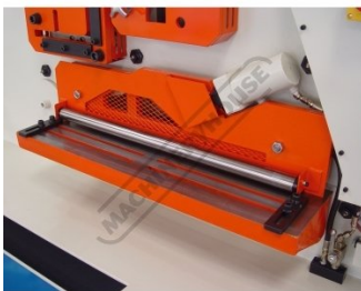
Includes Hydraulic Holddown for Flat Shear
