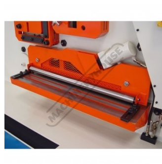
Optional Hydraulic Holddown for Flat Shear
