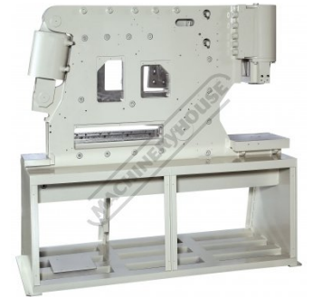
Monoblock Design For Rigid Frame Structure
