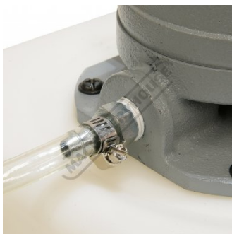
Coolant Pump Flow Outlet
