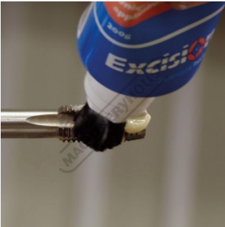
Tapping Application Close Up
