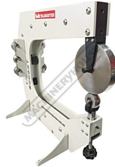
Wheels Set Parallel to Frame for those longer projects
