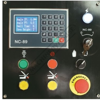
NC 89 Control Panel
