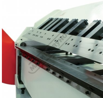
Shown with Material Clamp Beam Open
