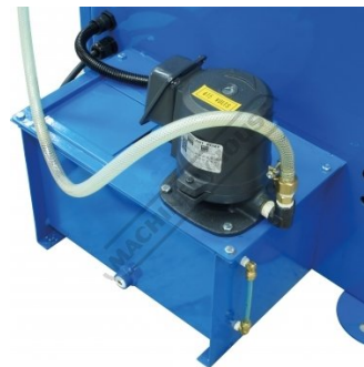
Coolant Pump and Tank
