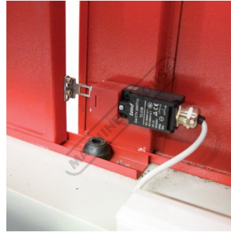
Rear Doors Safety Micro Switch
