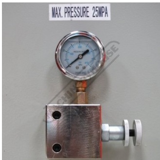
Adjustable Pressure Control
