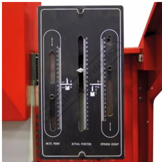
Adjustable Travel Limit Control
