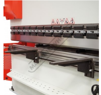
Adjustable and Sliding Front Sheet Supports
