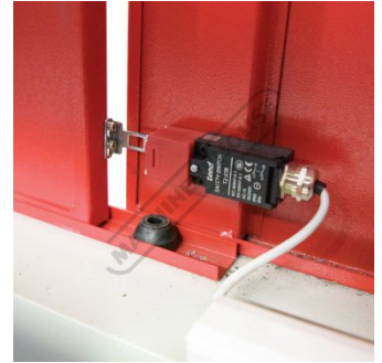
Rear Doors Safety Micro Switch
