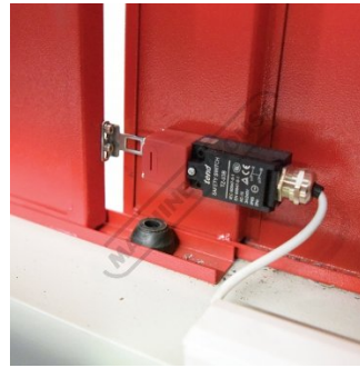
Rear Doors Safety Micro Switch
