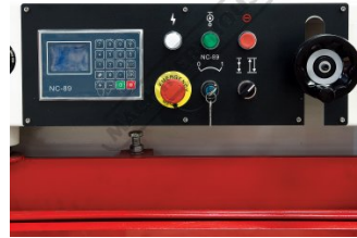
NC 89 Control Panel
