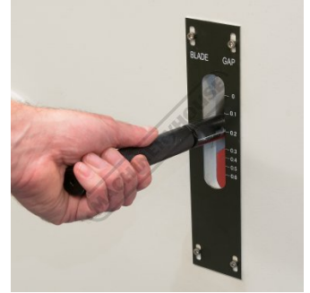
Quick Action Blade Clearance Adjustment Operation
