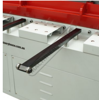
Front Sheet Supports with Roller Bearings
