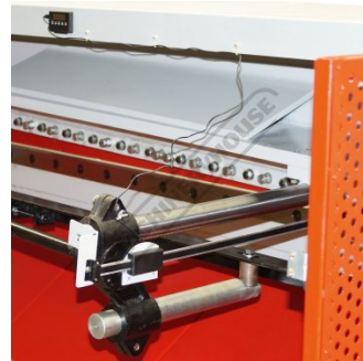
Backgauge with Digital Readout
