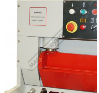
Spring Assisted Material Clamp Bar
