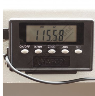
Backgauge Digital Readout
