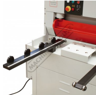
Squaring Arm with Measuring Scale
