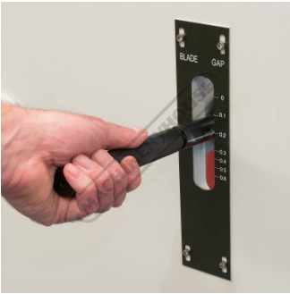
Quick Action Blade Clearance Adjustment Operation
