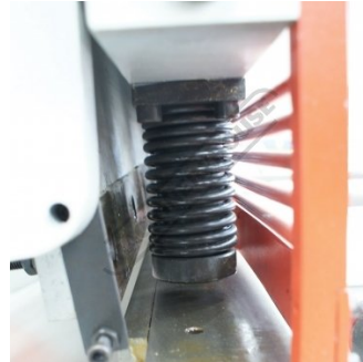
Hydraulic Material Hold Downs
