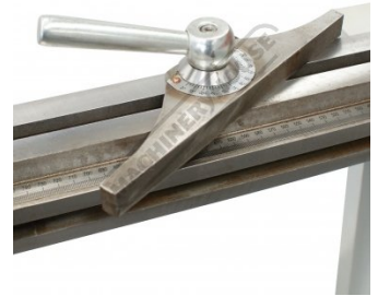
Adjustable and sliding mitre guide
