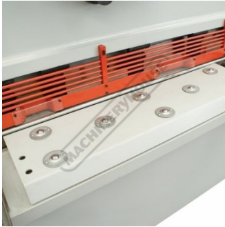
Material transfer balls on the table
