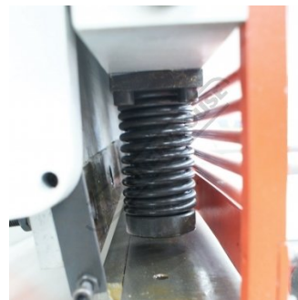
Hydraulic material hold downs
