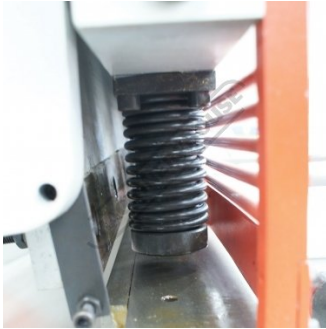
Hydraulic material hold downs
