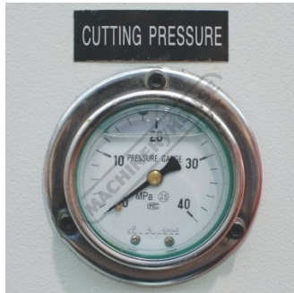
Cutting Pressure Gauge
