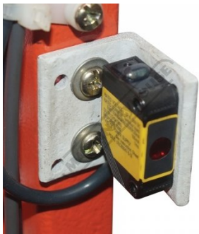
Safety Omron E3ZS Rear Light Sensor Guarding
