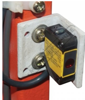
Safety Omron E3ZS Rear Light Sensor Guarding
