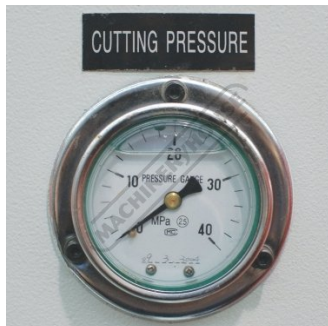
Cutting Pressure Gauge
