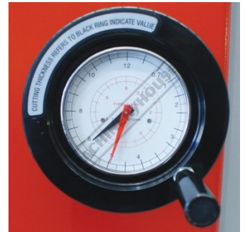
Variable Blade Gap Adjustment Dial
