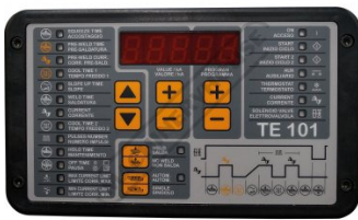
Control Panel TE101
