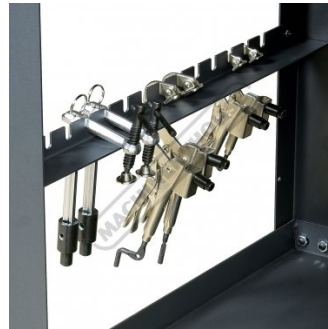
Storage Rack for Clamps Rear View
