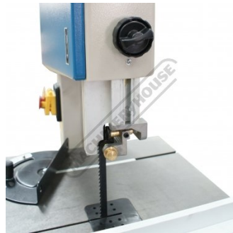
Height Adjustment handle for Top Blade Guide
