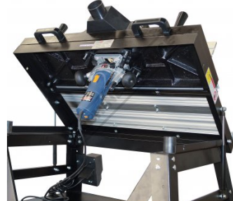
Mounting a Suitable Router
