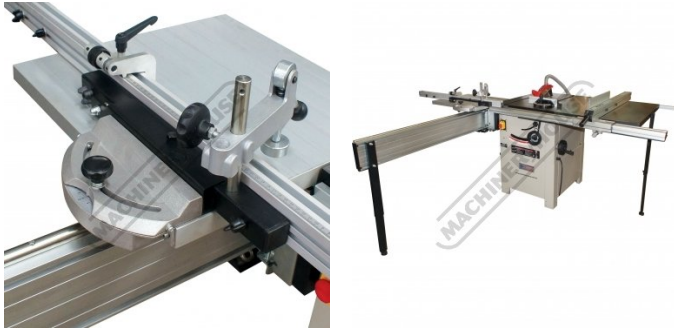
Material Clamp with Adjustable Guide Shown With Optional Table Saw
