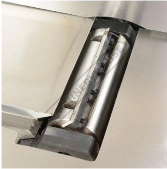
3 Blade Cutter Head
