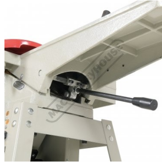
In-Feed Table Height Adjustment
