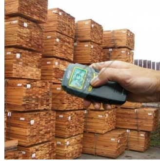
Measuring Moisture Content in Wood
