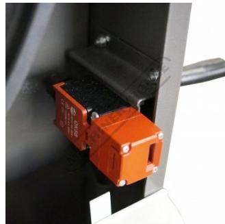
Safety Electrical Cut Out On Doors
