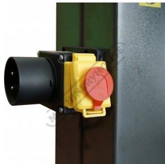
Electrical Emergency Stop
